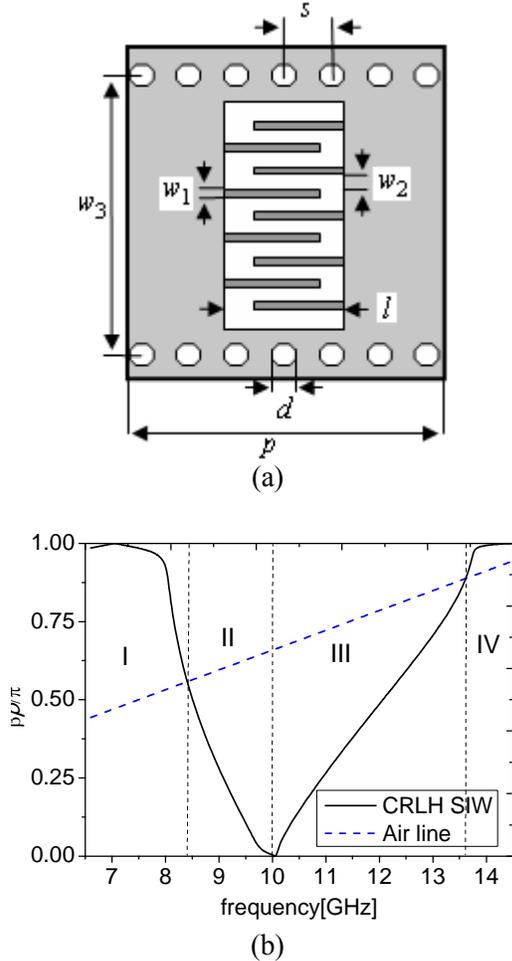
Fig. 1. (a) CRLH unit cell. The parameters are:  $w_1=0.33\text{mm}$ ,  $w_2=0.45\text{mm}$ ,  $w_3=9.2\text{mm}$ ,  $p=8.2\text{mm}$ ,  $l=3.3\text{mm}$ ,  $d=0.8\text{mm}$ ,  $s=1.45\text{mm}$ , and  $n=9$  (number of fingers). (b) Dispersion diagram of the unit cell (I. LH guided wave region, II. LH radiation region, III. RH radiation region and IV. RH guided wave region).
