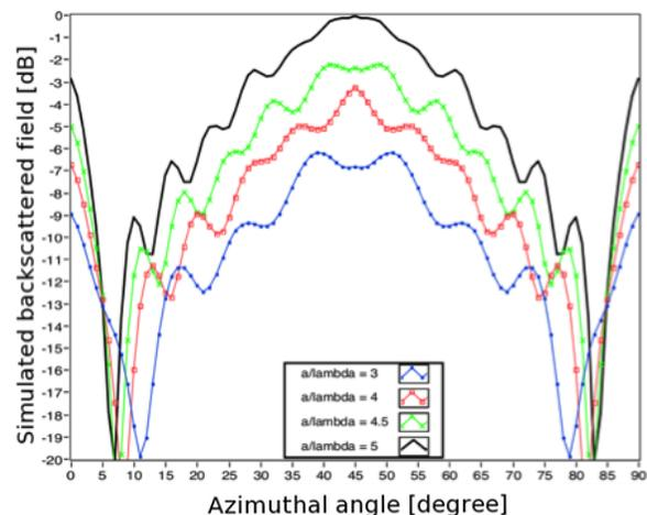
Fig. 1. Simulated dihedral backscattering for different dihedral dimensions. The graph shows the backscattered field (in dB) versus the azimuthal angle (0, 90°). The blue curve is relative to  $a/\lambda = 3$ ; the red curve is relative to  $a/\lambda = 4$ ; the green curve is relative to  $a/\lambda = 4.5$ ; finally, the black curve is relative to  $a/\lambda = 5$ . The different curves are separated of 6, 4, 2 dB, respectively, from the black one.
