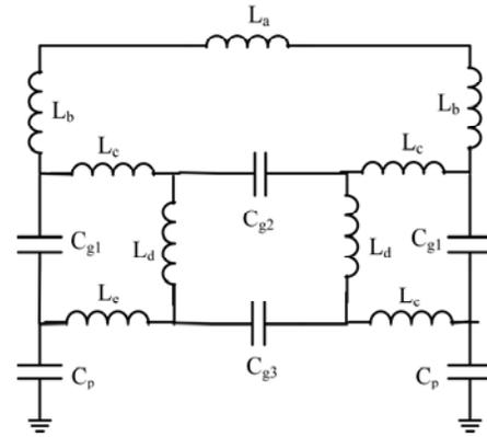
Fig. 2. LC equivalent circuit of the proposed resonator.
