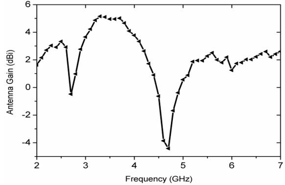
Fig. 14. Measured peak gain of the proposed antenna.
