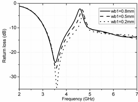
Fig. 5. Simulated return loss for different  $wb1$ .
