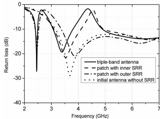
Fig. 3. Simulated return losses for the different structures.
