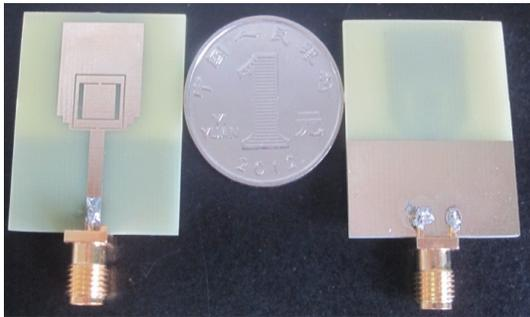
Fig. 2. Photograph of the proposed triple band antenna.
