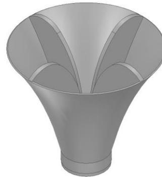
Fig. 8. Modelling of the quad-ridged horn.
