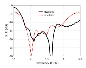
Fig. 8. The reflection coefficients of the proposed DRA.
