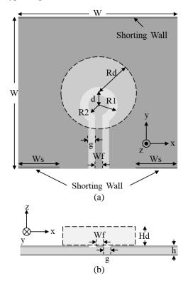
Fig. 1. The geometry of proposed wideband GCPW fed DRA: (a) top view and (b) side view.
