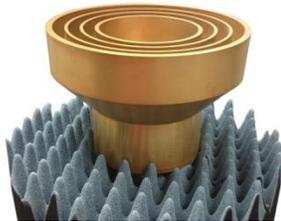
Fig. 2. Realised WR430 CATR feed.
