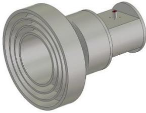
Fig. 1. Model of WR430 CATR feed.
