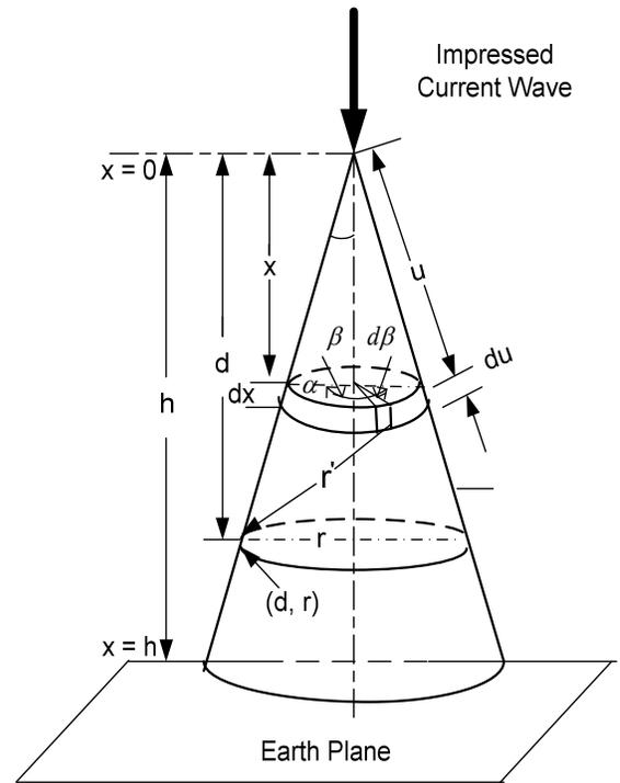
Fig. 5. Conical tower used in field theory analyses.
