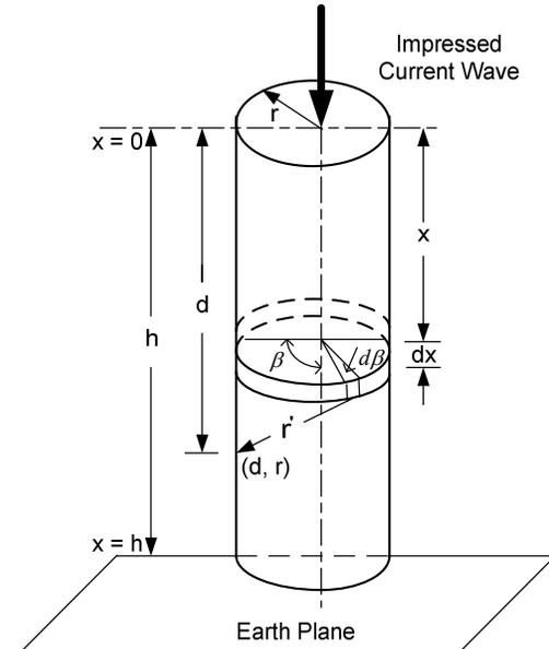
Fig. 4. Cylindrical tower used in field theory analyses.
