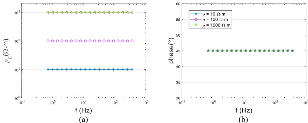
Fig. 5. WEM apparent resistivity (a) and phase (b) calculated for the homogeneous models. The transmit frequency is  $2^n$  Hz,  $n = -0.5:0.5:8.5$ , and the interval is 0.5, and the observation azimuth is 10 degrees.
