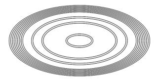
Fig. 5. Planar concentric coil with  $N_{ext} = 8$  and  $N_{int} = 3$ .
