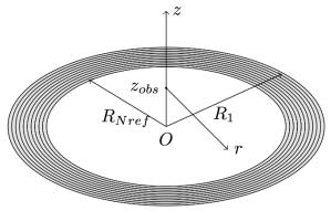
Fig. 2. Reference coil with all loops at the utmost exterior.
