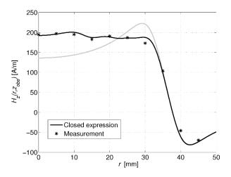
Fig. 9. Vertical magnetic field of the optimized coil at the observation height  $z_{obs}$  of 5 mm. The gray line shows the vertical magnetic field for the reference coil as comparison.
