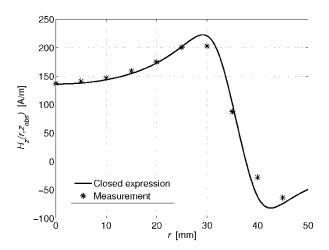
Fig. 7. Vertical magnetic field of the reference coil at the observation height  $z_{obs}$  of 5 mm.
