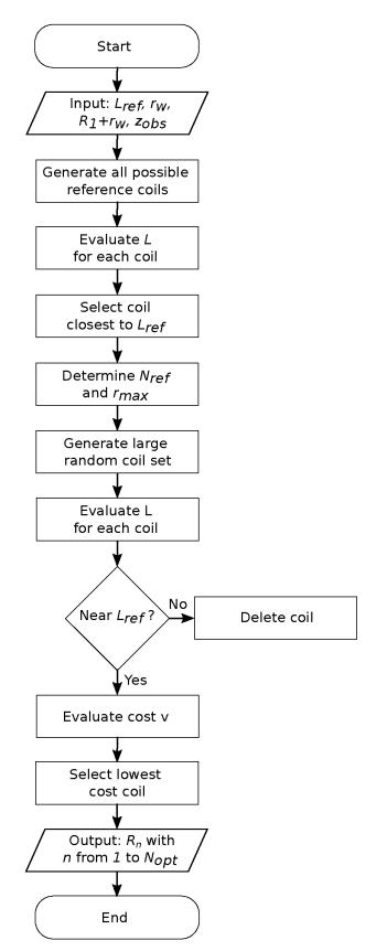
Fig. 4. Flowchart of the algorithm.
