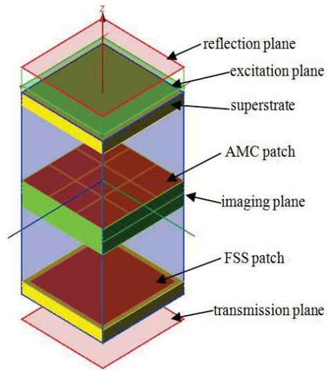
Fig. 3. Configuration of periodic imaging.
