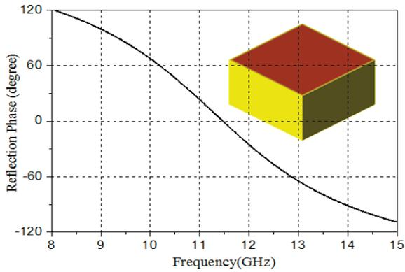
Fig. 1. Reflection phase of the patch AMC.
