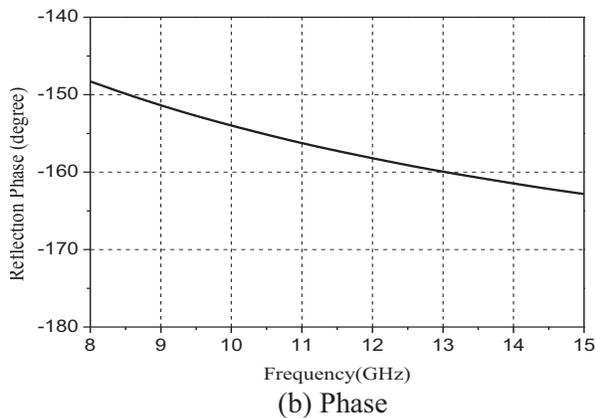
Fig. 2. Reflection characteristics of the patch FSS.
