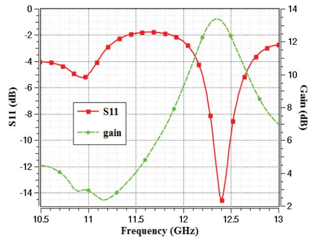
Fig. 7. Performance of cavity 1 with one dipole.
