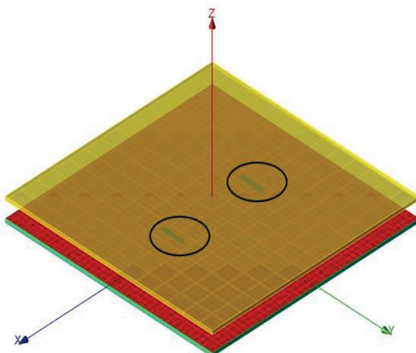
Fig. 9. Configuration of the F-P antenna with two dipoles.
