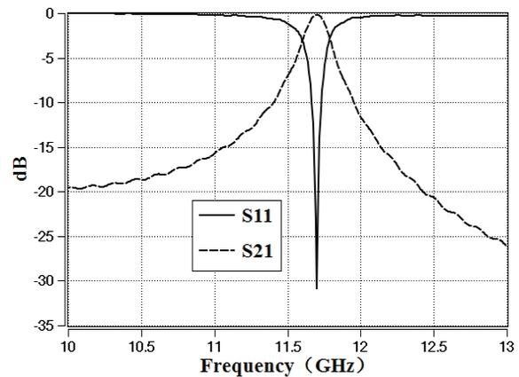
Fig. 4. S-parameters of the F-P cavity.
