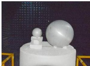
Fig. 15. The test double-PEC spheres.
