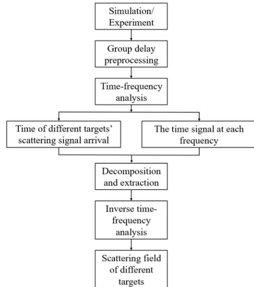
Fig. 1. The steps of extraction and recovery of scattering characteristics.
