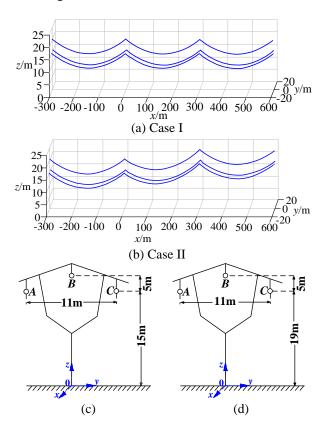
Fig. 3. Structure diagram of transmission line conductors.
