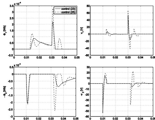
Fig. 4. Voltage switching rule with zero-bias and control laws (23) and (25) for  $k_1=0.92$ ,  $k_2=9.94$ .
