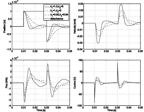
Fig. 2. Responses of closed-loop system with zero-bias to disturbances employing control law (23) for selected gains  $k_1$  and  $k_2$ .
