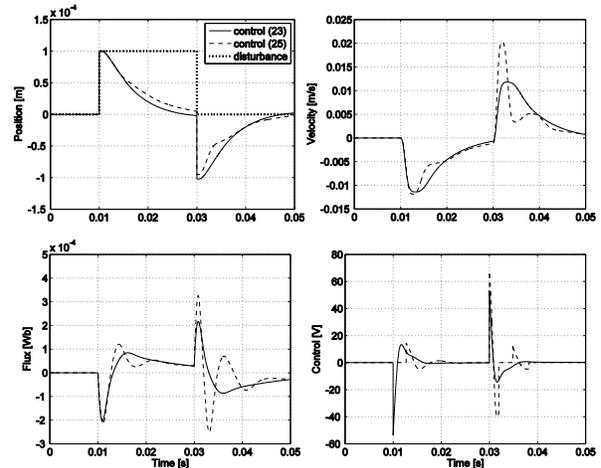
Fig. 3. Comparison of step responses between closed-loop systems employing (23) and (25) controllers for  $k_1=0.92, k_2=9.94$  with zero-bias.
