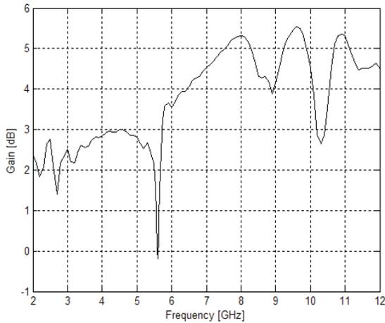
Fig. 6. Simulated gain of the proposed antenna.
