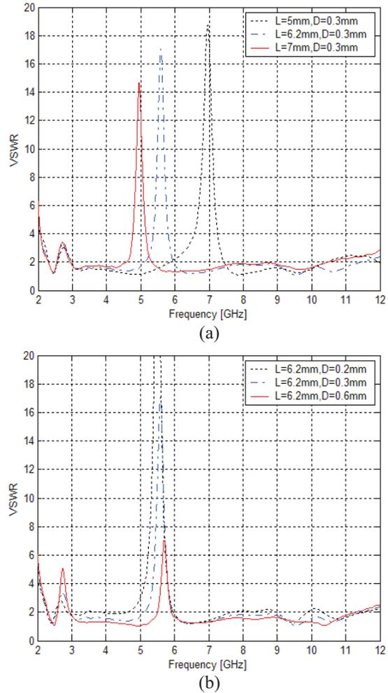
Fig. 2. Simulated VSWR with different: (a)  $L$ , and (b)  $D$ .
