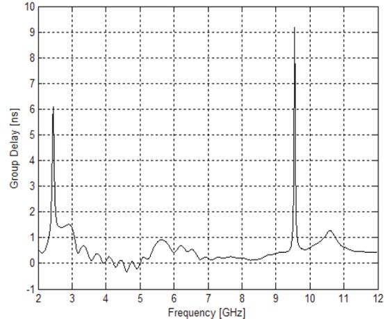
Fig. 8. Simulated group delay of the proposed antenna.
