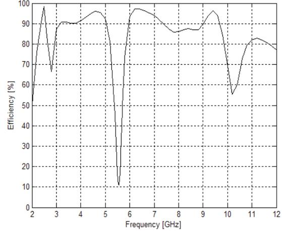
Fig. 7. Simulated efficiency of the proposed antenna.
