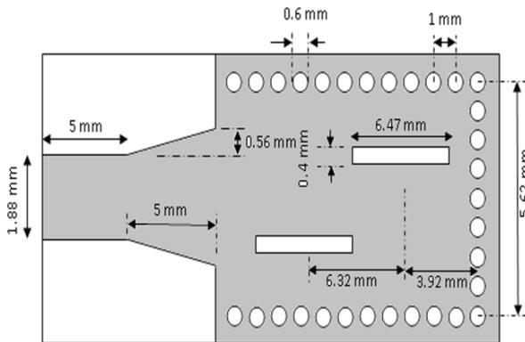
Fig. 4. Dimension for 2 slot SIW array antenna.
