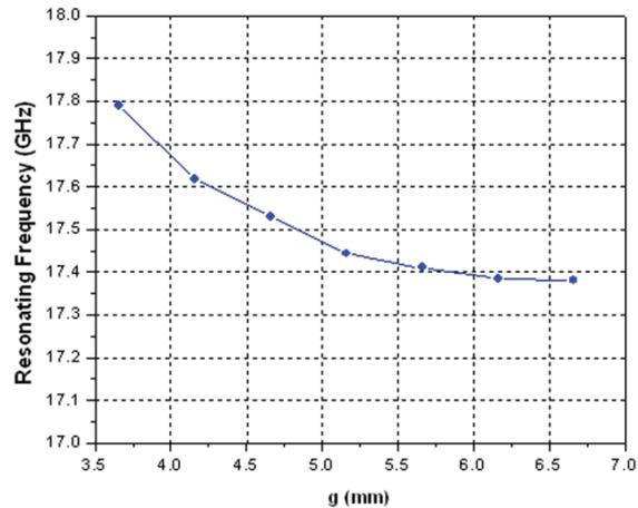
Fig. 16. Effect of slot position from end wall  $g$  on resonating frequency (measured).
