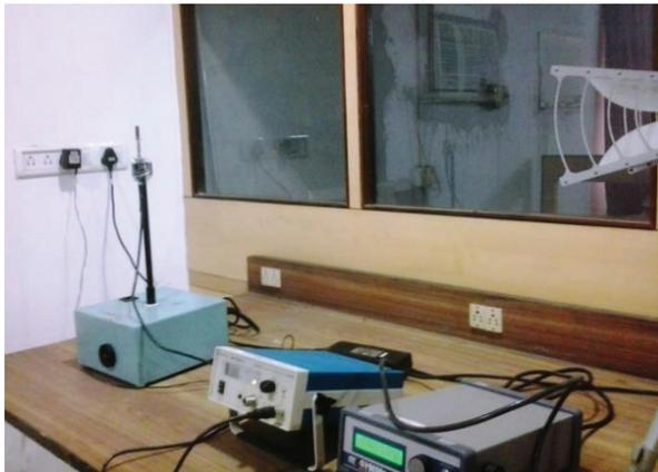
Fig. 9. Experimental set-up for radiation pattern measurement.
