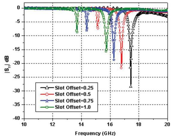
Fig. 7. Parametric analysis of several slot offset gap ( $p$ ).
