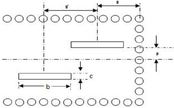
Fig. 3. Slot dimensions and gap between slots.
