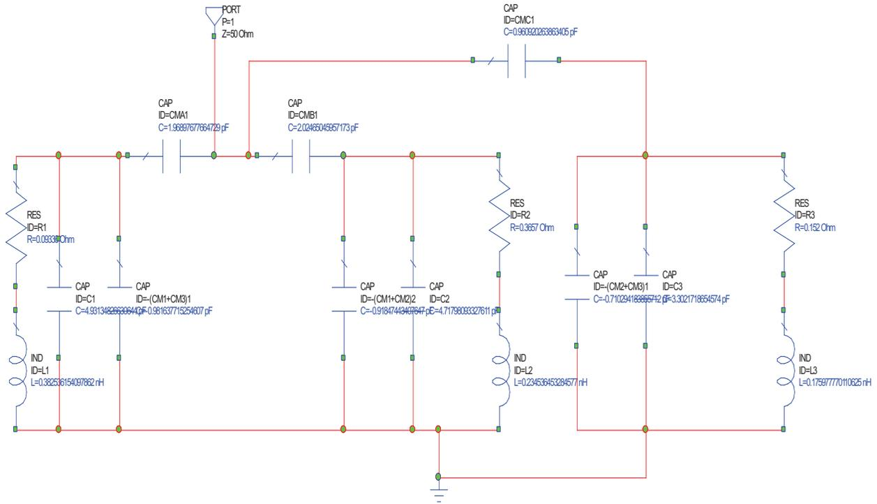
Fig. 8. Circuit model of triple band absorber.
