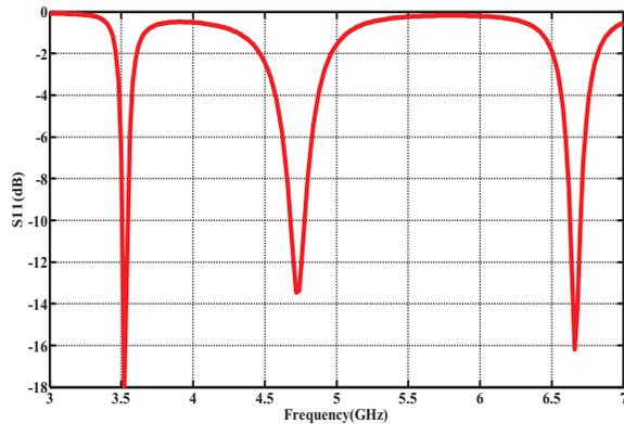
Fig. 9. S-parameter of simulated circuit model.
