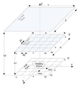
Fig. 1. Geometry of the problem, comprising the plane of radiating current sources at the location of PCB (z = 0), the measurement plane in the near filed zone ( $z = h_1$ ) and the far-field plane ( $z = h_2$ ) with unknown magnetic field distribution.
