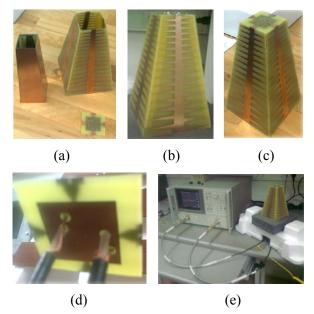
Fig. 8. The volume-confined PLPAs; (a) parts: four -arm radiator, conductive shield, and planar feeding circuit, (b), (c) views of the fabricated prototypes, (d) transmission line cables of the feeding system (internal side), and (e) measurement setup.
