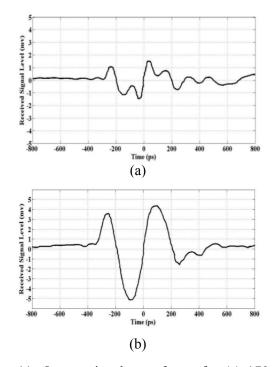
Fig. 11. Output signal waveforms for (a) 170 ps and (b) 280 ps input pulses.
