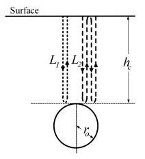
Fig. 3. Expected reflections from a buried cylindrical object.
