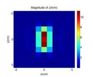
Fig. 13. Variations of the equivalent current (|J|) on the PCB plane (z = 0) predicted by the proposed model, using the data shown in Fig. 12.
