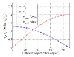
Fig. 4. Contrast of the magnetic charge density on pipe's side and end surfaces under different directions of magnetization.
