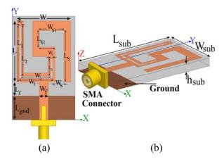
Fig. 1. Geometry of the proposed antenna, (a) top view and (b) side view.
