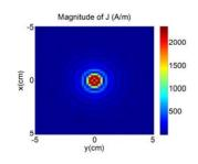
Fig. 5. Variations of the equivalent current (|J|) on the PCB plane (h = 0) predicted by the proposed model, using the data shown in Fig. 4.
