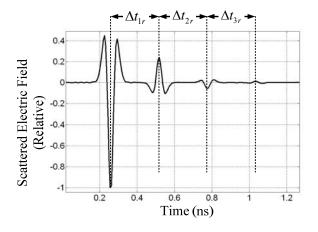
Fig. 7. TM<sub>z</sub> back scattered field from a buried cylindrical PEC object for  $r_a = 0.01$  m,  $h_c = 0.01$  m, wl = 2 m,  $x_c / r_a = 0.0$ ,  $\varepsilon_1 = 15 \varepsilon_0$  F/m,  $\mu_1 = \mu_0$  H/m,  $\phi_i = \phi_s = 90^{\circ}$ , and  $\sigma_1 = 0.001$  Sm<sup>-1</sup>.
