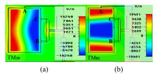
Fig. 2. Simulated electrical field amplitude distributions: (a)  $TM_{10}$  mode and (b)  $TM_{02}$  mode.
