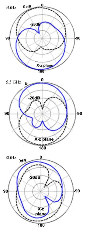
Fig. 5. Measured radiation patterns of the proposed antenna.
