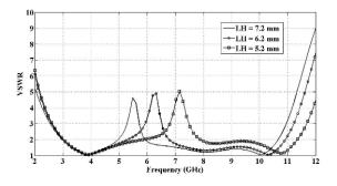
Fig. 4. Simulated VSWR characteristics for different values of  $L_{\rm H}$  (g = 0.2 mm).
