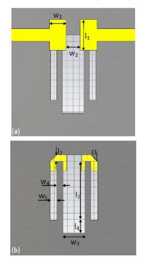
Fig. 11. 2D view of the new SGS BPF; (a) top and (b) bottom layers.
