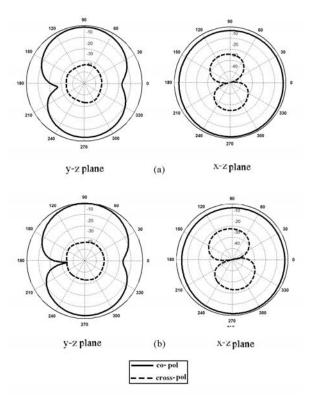
Fig. 11. Measured radiation patterns of the proposed antenna at (a) 5.2 GHz and (b) 5.8 GHz.
