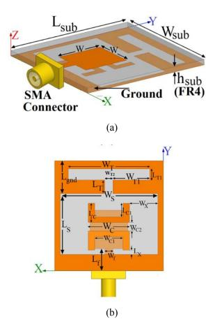
Fig. 1. Geometry of the proposed square slot antenna; (a) bottom view and (b) side view.
