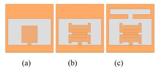
Fig. 2. (a) The ordinary square slot antenna, (b) antenna with a pair of U-shaped parasitic structures in the ground plane, and (c) the proposed square slot antenna.
