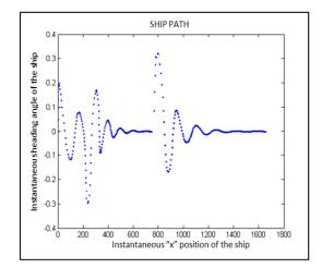
Fig. 9. Instantaneous turning rate of the ship (Integrated System).
