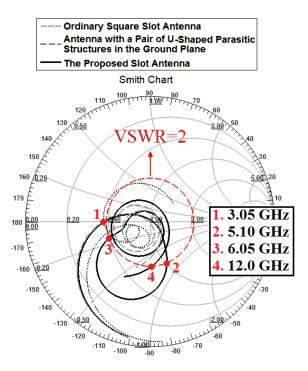
Fig. 4. The simulated input impedance on a Smith chart for the various slot antenna structures shown in Fig. 2.
