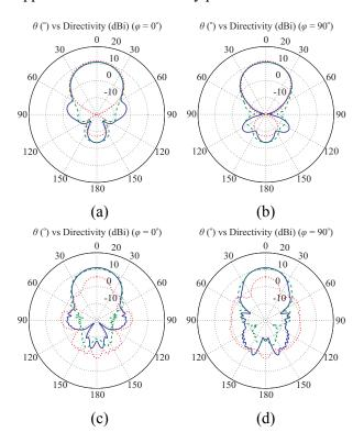
Fig. 15. Radiation patterns of diverse PLPAs with Euclidean (blue continuous line), 2nd-order meander (green dashed line), and 3rd-order meander (red dotted line) elements at (a), (b) f = 20 GHz, and (c), (d) f = 100 GHz.
