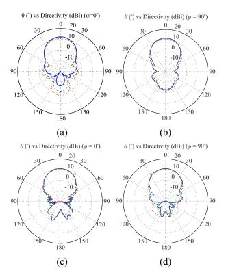
Fig. 7. Radiation patterns of different PLPAs with  $\tau_a = 20^{\circ}$  (blue continuous line),  $\tau_a = 25^{\circ}$  (green dashed line), and  $\tau_a = 30^{\circ}$  (red dotted line) at (a), (b) f = 20 GHz and (c), (d) f = 100 GHz.
