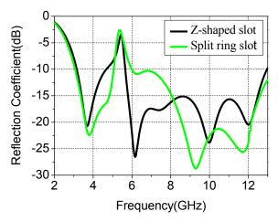
Fig. 3. Simulated reflection coefficient of a single notched slot.
