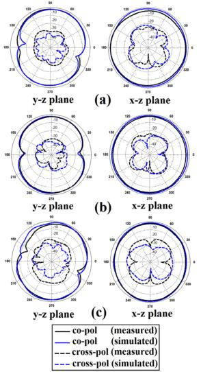
Fig. 8. Measured and simulated radiation patterns of the proposed antenna at (a) 4 GHz, (b) 7 GHz, and (c) 10 GHz.
