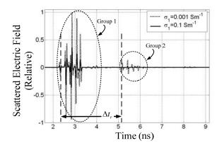
Fig. 13. TM<sub>z</sub> back scattered field from a buried cylindrical PEC object for  $r_a = 0.01$  m,  $h_c = 0.1$  m, wl = 2 m,  $x_c / r_a = 0.0$ ,  $\varepsilon_1 = 15 \varepsilon_0$  F/m,  $\mu_1 = \mu_0$  H/m,  $\phi_i = \phi_s = 20^0$ ,  $w_p = 0.1$  m, and  $h_p/w_p = 0.1$ .
