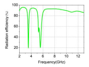
Fig. 7. Simulated radiation efficiency of the proposed band-notched antenna.
