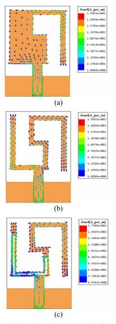
Fig. 5. Simulated surface current distributions on the radiating patch for antennas shown in Fig. 2 at (a) first resonance frequency (1.8 GHz), (b) second resonance frequency (2.4 GHz), and (c) third resonance frequency (3.5 GHz).
