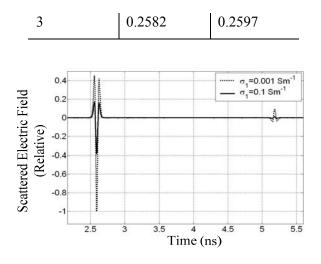
Fig. 8. TM<sub>z</sub> back scattered field from a buried cylindrical PEC object for  $r_a = 0.01$  m,  $h_c = 0.1$  m, wl = 2 m,  $x_c / r_a = 0.0$ ,  $\varepsilon_1 = 15 \varepsilon_0$  F/m,  $\mu_1 = \mu_0$  H/m, and  $\phi_i = \phi_s = 90^0$ .
