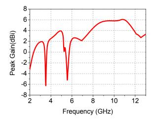
Fig. 6. Simulated gain curve of the proposed bandnotched antenna.
