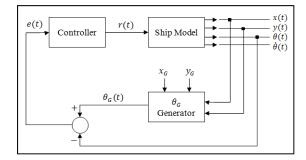
Fig. 5. Block diagram of the PID control system.
