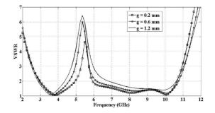
Fig. 5. Simulated VSWR characteristics for different values of g ( $L_{\rm H}$  = 7.2 mm).
