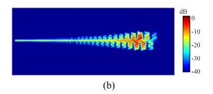
Fig. 16. Surface current density of two volumeoptimized meander-toothed PLPAs; (a) 2nd-order at f = 40 GHz and (b) 3rd-order at f = 20 GHz.
