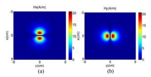
Fig. 4. Variations of the tangential magnetic field produced by the electrical loop on the near-field plane ( $h_1 = 10 \text{ mm}$ ); (a)  $H_x$  and (b)  $H_y$ .
