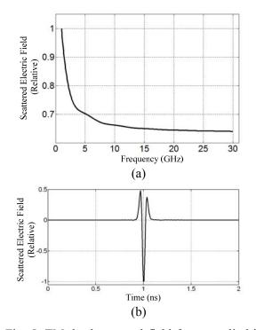
Fig. 4. The incident E-field waveform (a) in frequency and (b) time domains.
