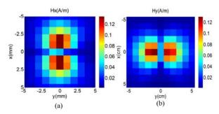
Fig. 8. Variations of the measured tangential magnetic field produced by the high frequency inductor on the near-field plane ( $h_1 = 10$  mm); (a)  $H_x$  and (b)  $H_y$ .
