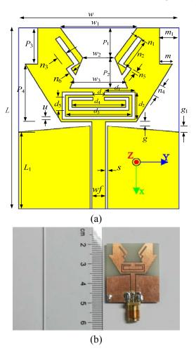
Fig. 1. (a) Geometry of the proposed antenna and (b) photograph of the proposed antenna.
