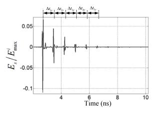
Fig. 10. TM<sub>z</sub> back scattered field from a buried cylindrical PEC object for  $r_a = 0.01$  m,  $h_c = 0.02$  m, wl = 2 m,  $x_c / r_a = 0.0$ ,  $\varepsilon_1 = 15 \varepsilon_0$  F/m,  $\mu_1 = \mu_0$  H/m,  $\phi_i = \phi_s = 90^{\circ}$ ,  $w_p = 0.1$  m,  $h_p/w_p = 0.1$ , and  $\sigma_1 = 0.001$  Sm<sup>-1</sup>.
