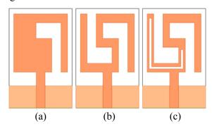
Fig. 2. (a) The ordinary square antenna with an L-shaped slit in the radiating patch, (b) the antenna with a pair of L-shaped slits in the radiating patch, and (c) the proposed antenna.
