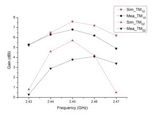
Fig. 9. Simulated and measured gains of the proposed antenna versus frequency.
