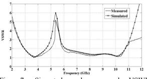
Fig. 7. Simuated and measured VSWR characteristics for the fabricated antenna.
