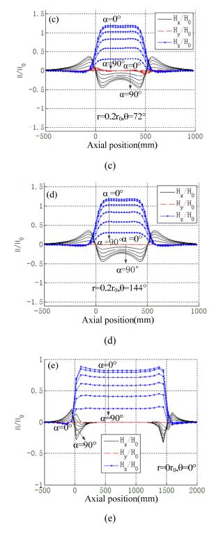
Fig. 6. Magnetic field distributions in different pipes under different directions of magnetization;  $\alpha = 0^{\circ}$ , 15°, 30°, 45°, 60°, 75°, 90°;  $r_0 = 100$  mm, t = 7 mm, (a)-(d)  $l_0 = 500$  mm and (e)  $l_0 = 1500$  mm.
