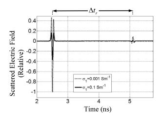
Fig. 9. TM<sub>z</sub> back scattered field from a buried cylindrical PEC object for  $r_a = 0.01$  m,  $h_c = 0.1$  m, wl = 2 m,  $x_c / r_a = 0.0$ ,  $\varepsilon_1 = 15 \varepsilon_0$  F/m,  $\mu_1 = \mu_0$  H/m,  $\phi_i = \phi_s = 20^0$ , and  $\sigma_1 = 0.001$  Sm<sup>-1</sup>.
