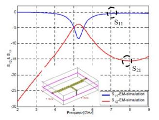
Fig. 4. Simulation results of the first proposed band pass filter (structure 1).
