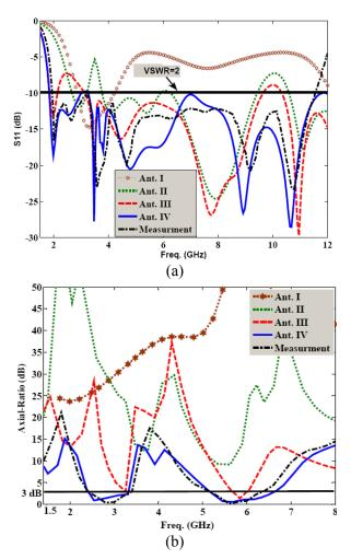
Fig. 2. Measured and simulated  $S_{11}$  and CP axial ratios for Ants. I to IV.
