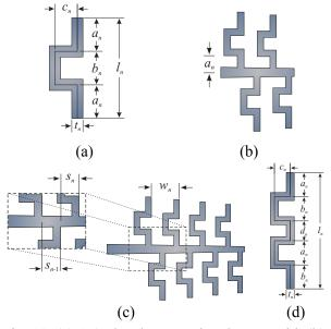
Fig. 10. (a) A 2nd-order meander element with (b), (c) its main design parameters, and (d) a 3rd-order meander element.
