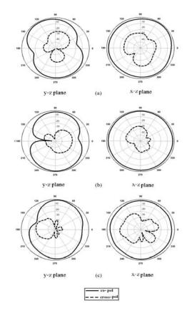
Fig. 10. Measured radiation patterns of the proposed antenna at (a) 4 GHz, (b) 7 GHz, and (c) 10 GHz.
