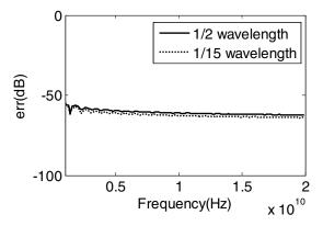
Fig. 3. Variation of the reflection relative error of the PSTD-CPML method with respect to frequency.
