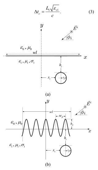
Fig. 2. The medium with (a) flat surface and (b) sinusoidal surface.
