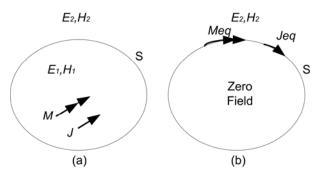
Fig. 2. The electromagnetic equivalence principle; (a) the original problem and (b) the equivalent problem.
