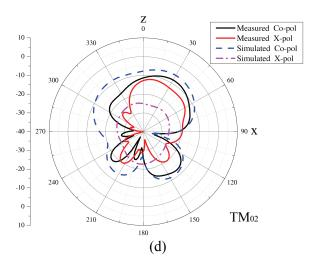
Fig. 8. Simulated and measured radiation patterns at 2.45 GHz: (a)  $TM_{10}$  mode in the *y*-*z* plane, (b)  $TM_{02}$  mode in the *y*-*z* plane, (c)  $TM_{10}$  mode in the *x*-*z* plane, and (d)  $TM_{02}$  mode in the *x*-*z* plane.
