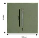
Fig. 11. Microstrip transmission line.
