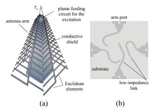
Fig. 2. The four-arm PLPA with Euclidean elements and a pyramidal grounded conductive shield for (a) perspective view and (b) planar feeding circuit.
