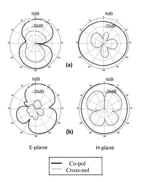
Fig. 8. Measured E-plane and H-plane radiation patterns for the proposed antenna at (a) 3.5 GHz and (b) 9.5 GHz.
