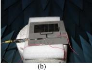
Fig. 7. (a) Photograph of the fabricated antenna and (b) photograph of the proposed antenna in a spherical near-field measurement system.
