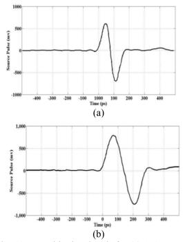
Fig. 10. Input bipolar signals for (a) 170 ps and (b) 280 ps.
