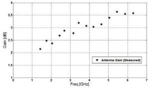
Fig. 8. Measured maximum gain and simulated radiation efficiency values of the proposed monopole antenna.
