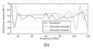
Fig. 14. Comparison between various PLPAs with different elements; (a) directivity and (b) half-power beamwidth.
