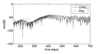
Fig. 2. The reflection relative error of the CPML with  $\Delta t = 112.5$  ps.
