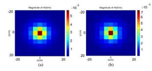
Fig. 10. Variations of the tangential magnetic field  $(\sqrt{H_x^2 + H_y^2})$  produced by high frequency inductor on the far-field plane ( $h_2 = 50$  mm); (a) reconstructed and (b) measured results.
