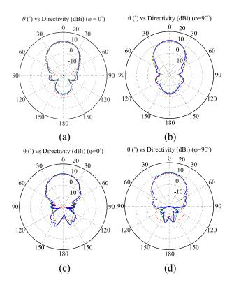
Fig. 4. Radiation patterns of various PLPAs with  $t_n$ =  $0.5s_n$  (blue continuous line),  $t_n = 0.2s_n$  (green dashed line), and  $t_n = 0.05s_n$  (red dotted line) at (a), (b) f = 20 GHz and (c), (d) f = 100 GHz.
