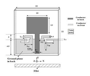
Fig. 1. Geometry of the proposed antenna.
