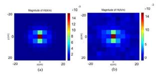
Fig.14. Variations of the tangential magnetic field  $(\sqrt{H_x^2 + H_y^2})$  produced by micro strip transmission line on the far-field plane ( $h_2$ =50mm); (a) reconstructed and (b) measured results.
