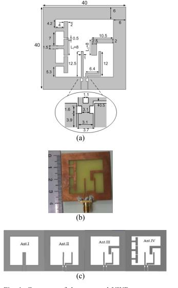
Fig. 1. Geometry of the proposed UWB antenna; (a) antenna configuration, (b) photo of the optimized antenna, and (c) four prototypes of the CPSSA under investigation.
