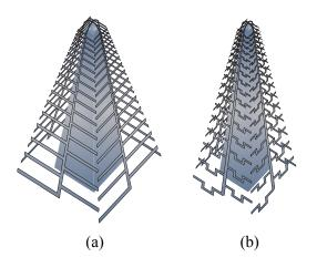
Fig. 11. Geometry of (a) the Euclidean-element and (b) the proposed meander-element PLPA.
