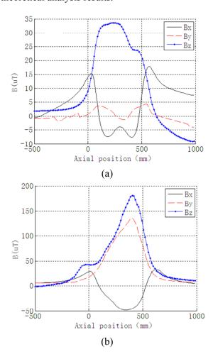
Fig. 9. Measured magnetic induction intensity inside pipes; (a)-(c)  $l_0 = 500$  mm and (d)  $l_0 = 1500$  mm.
