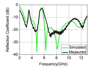
Fig. 4. Simulated and measured reflection coefficient of the proposed antenna.
