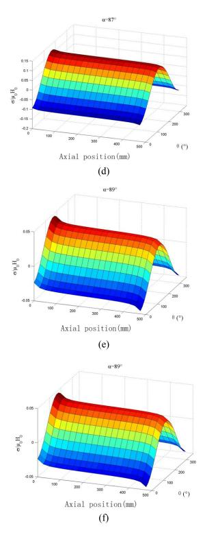
Fig. 5. Magnetic charge density distributions on pipe's outer side surface under different directions of magnetization.
