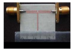
Fig. 7. Photograph of the fabricated optimized band pass filter.
