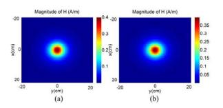
Fig. 6. Variations of the tangential magnetic field  $(\sqrt{H_x^2 + H_y^2})$  produced by the electrical loop on the far-field plane ( $h_2 = 50$  mm); (a) theoretical and (b) reconstructed results.
