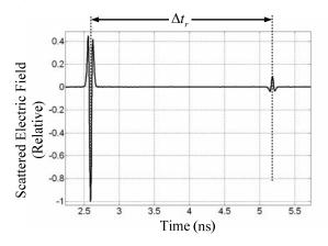
Fig. 6. TM<sub>z</sub> backscattered field from a buried cylindrical PEC object for  $r_a = 0.01$  m,  $h_c = 0.1$  m, wl = 2 m,  $x_c / r_a = 0.0$ ,  $\varepsilon_1 = 15 \varepsilon_0$  F/m,  $\mu_1 = \mu_0$  H/m,  $\phi_i = \phi_s = 90^{\circ}$ , and  $\sigma_1 = 0.001$  Sm<sup>-1</sup>.
