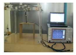
Fig. 3. Experimental setup for magnetic field measurements.
