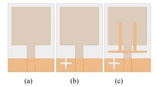
Fig. 2. (a) basic structure (ordinary monopole antenna), (b) antenna with a cross-shaped slit in the ground plane, and (c) the proposed antenna.
