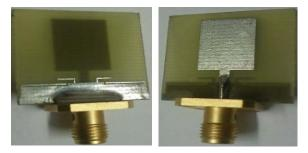
Fig. 6. Photographs of the manufactured antenna.
