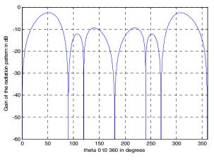
(b) Rectangular plot of the phase scanning array in dB.
