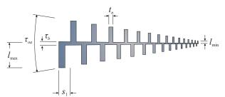
Fig. 1. Geometry of a Euclidean-toothed arm.
