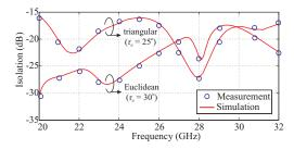
Fig. 9. Isolation of the fabricated triangular- and Euclidean-toothed volume-confined PLPAs.
