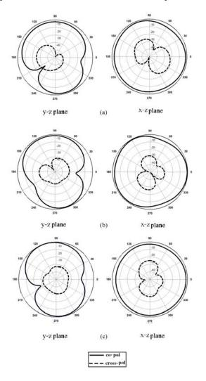
Fig. 10. Measured radiation patterns of the proposed antenna at (a) 1.8 GHz, (b) 2.4 GHz, and (c) 3.5 GHz.
