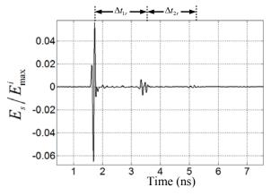
Fig. 11. TM<sub>z</sub> back scattered field from a buried cylindrical PEC object for  $r_a = 0.01$  m,  $h_c = 0.06$  m, wl = 2 m,  $x_c / r_a = 0.0$ ,  $\varepsilon_1 = 15 \varepsilon_0$  F/m,  $\mu_1 = \mu_0$  H/m,  $\phi_i = \phi_s = 90^{\circ}$ ,  $w_p = 0.1$  m,  $h_p/w_p = 0.1$ , and  $\sigma_1 = 0.001$  Sm<sup>-1</sup>.
