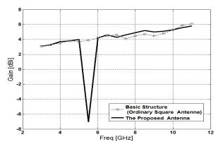
Fig. 11. Measured maximum gain comparisons for the ordinary square antenna and the proposed antenna.
