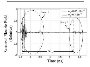
Fig. 12.  $\text{TM}_z$  back scattered field from a buried cylindrical PEC object for  $r_a = 0.01$  m,  $h_c = 0.1$  m, wl = 2 m,  $x_c / r_a = 0.0$ ,  $\varepsilon_1 = 15 \varepsilon_0$  F/m,  $\mu_1 = \mu_0$  H/m,  $\phi_i = \phi_s = 90^0$ ,  $w_p = 0.1$  m, and  $h_p/w_p = 0.1$ .
