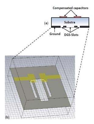
Fig. 10. 3D view of the new proposed SGS band pass filter (structure 5).
