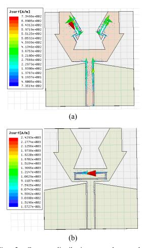
Fig. 2. Current distributions at the notched frequency.
