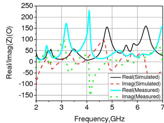
Fig. 4. Simulated and measured impedance of the antenna.
