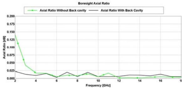
Fig. 5. Axial ratio comparison of the sinuous antenna, with and without back cavity.
