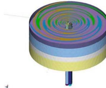
Fig. 8. Emerson and Cuming ECCOSORB AN absorbers loaded in back cavity.
