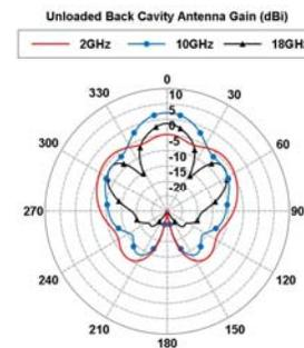
Fig. 7(a). Gain pattern of the sinuous antenna with the back cavity.
