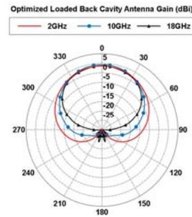
Fig. 9. Gain pattern of the optimized sinuous antenna.
