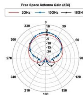
Fig. 7(b). Gain pattern of the sinuous antenna without the back cavity.
