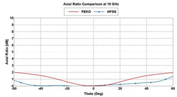
Fig. 17. Axial ratio comparison of the optimized sinuous antenna at 10 GHz.
