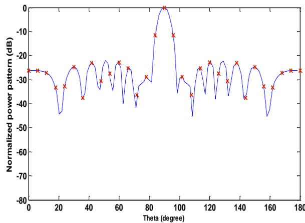
Fig. 9. Damaged array pattern with fault at 3<sup>rd</sup> and 19<sup>th</sup> sensors with 31 samples.
