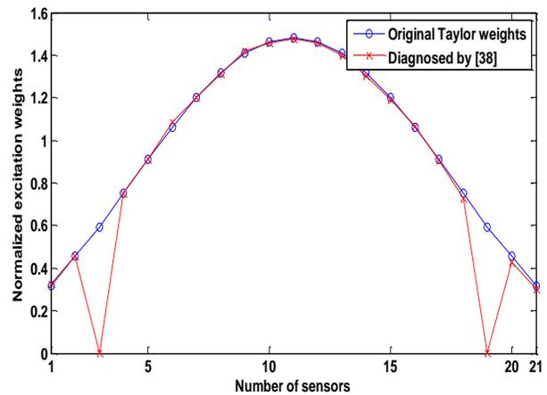
Fig. 12. Performance of the conventional method [38] with 16 samples.
