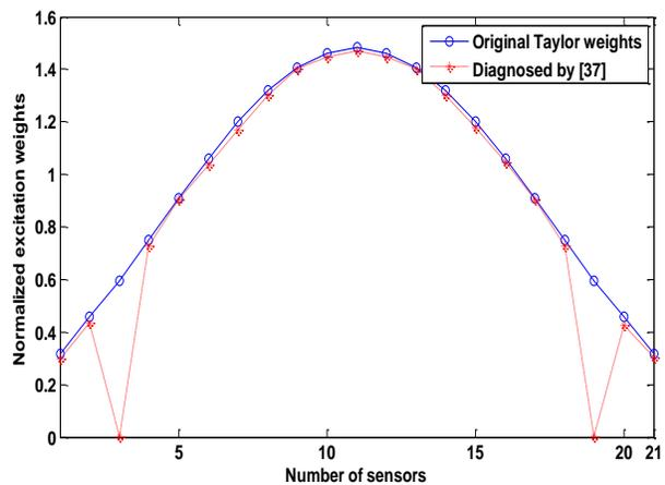
Fig. 10. Performance of the conventional method [37] with 31 samples.
