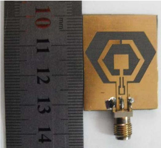
(a) Antenna 2 with two switches ON.
