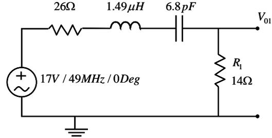
Fig. 3. Thevenin source with complex impedance loaded by resistance  $R_1$ .
