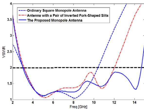
Fig. 3. Simulated VSWR characteristics for the various monopole antennas shown in Fig. 2.
