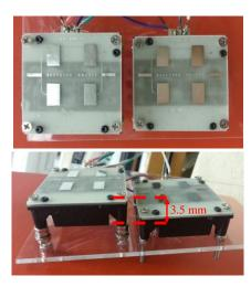
Fig. 3. Quadrature radar assembly is illustrated. A physical offset of approximately 3.5 mm has been kept between the two MDU1020 single channel k band radars [2].
