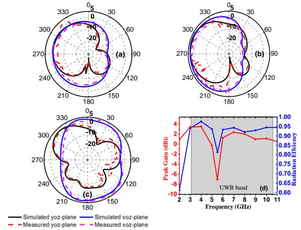
Fig. 7. Simulated and measured radiation pattern of UWB MIMO antenna at: (a) 4 GHz, (b) 7 GHz, (c) 10 GHz, and (d) measured peak gain and radiation efficiency of the proposed UWB MIMO antenna.
