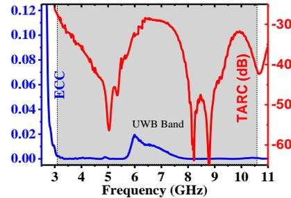
Fig. 8. Measured ECC and TARC of the proposed UWB MIMO antenna against frequency.
