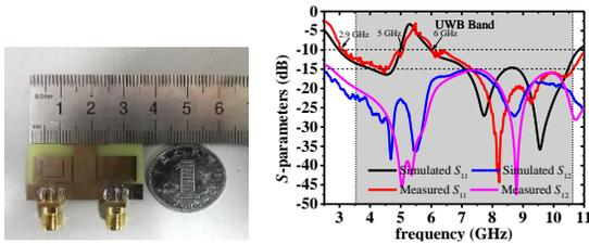
Fig. 6. The prototype and S-parameters of the UWB MIMO antenna
