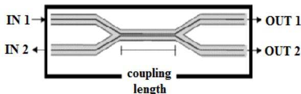
Fig. 1. The general model for directional couplers.
