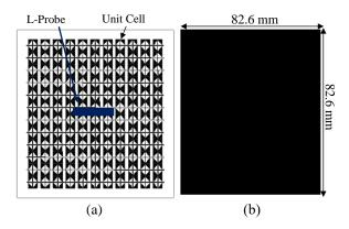
Fig. 3. (a) Top-view of the ground plane consisting of a  $12 \times 12$  unit cells. (b) Bottom-view of the ground plane consisting of a solid PEC metal plate.
