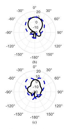
Fig. 6. Radiation patterns of the wideband AMC U-slot patch antenna at: (a) 3.2 GHz, (b) 3.9 GHz, and (c) 4.6 GHz; E-plane: solid black line, H-plane: dashed blue line.
