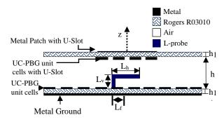
Fig. 1. Side-view of the wideband  $TE_{10}$  patch antenna with UC-PBG unit cells in both the patch and the ground plane excited by an L-probe with  $L_v$ =5.535 mm,  $L_h$ =15 mm,  $L_f$ =7mm, h=6.4mm, and h<sub>1</sub>=0.635mm.
