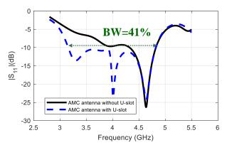
Fig. 4. Reflection coefficients of the AMC antenna exciting the  $TE_{10}$  mode with and without the U-slot.
