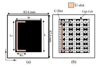
Fig. 2. (a) Top-view of the patch with PEC metal plate with a U-slot. (b) Bottom-view of the patch with unit cells and U-slot placed exactly below the PEC metal plate with dimensions of  $L \times W=46.2mm \times 26.4mm$ ; L<sub>s</sub>=46mm, W<sub>s</sub>=6mm.
