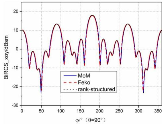
Fig. 3. Bistatic RCS of the cylinder arrays.
