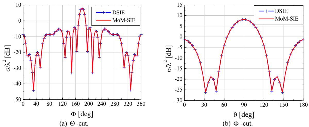
Fig. 10. RCS calculated using DSIE vs. classical MoM-SIE.
