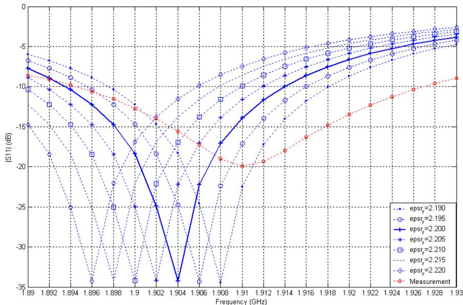
**Fig. 5** WIPL calculations showing the change in the resonant frequency when the substrate dielectric constant was varied over the tolerance range certified by the vendor.
