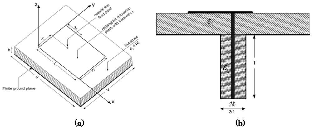
**Fig.1** Rectangular microstrip patch, (a), E-plane cut, (b)
