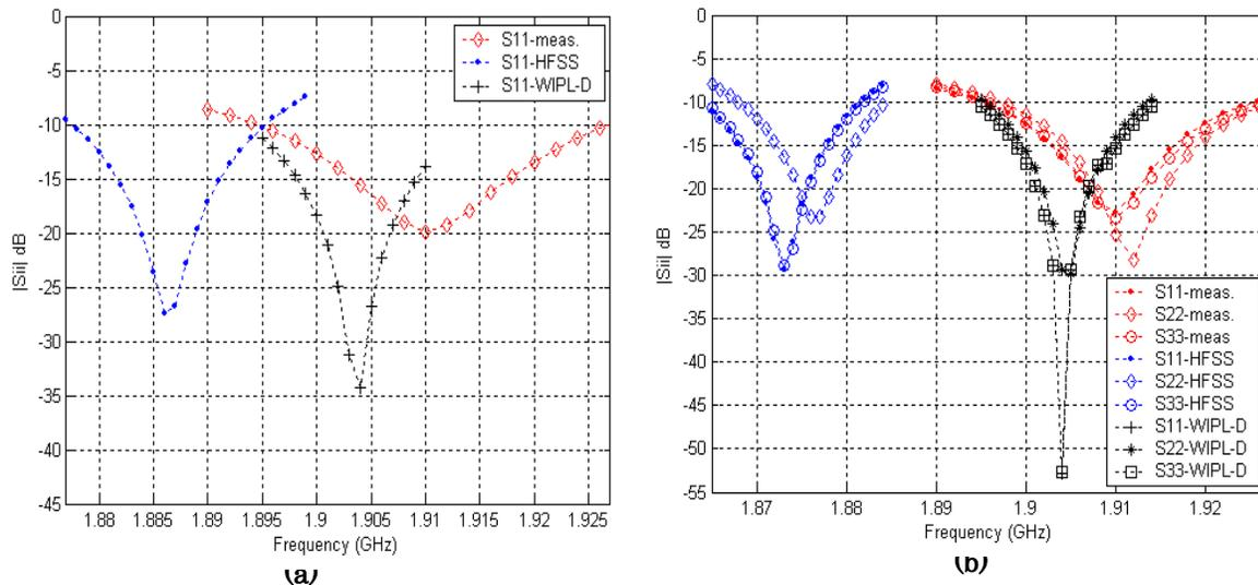
**Fig.4** Return loss predicted by WIPL-D and HFSS with for a single patch, (a), and 3-element patch, (b), compared with experiment
