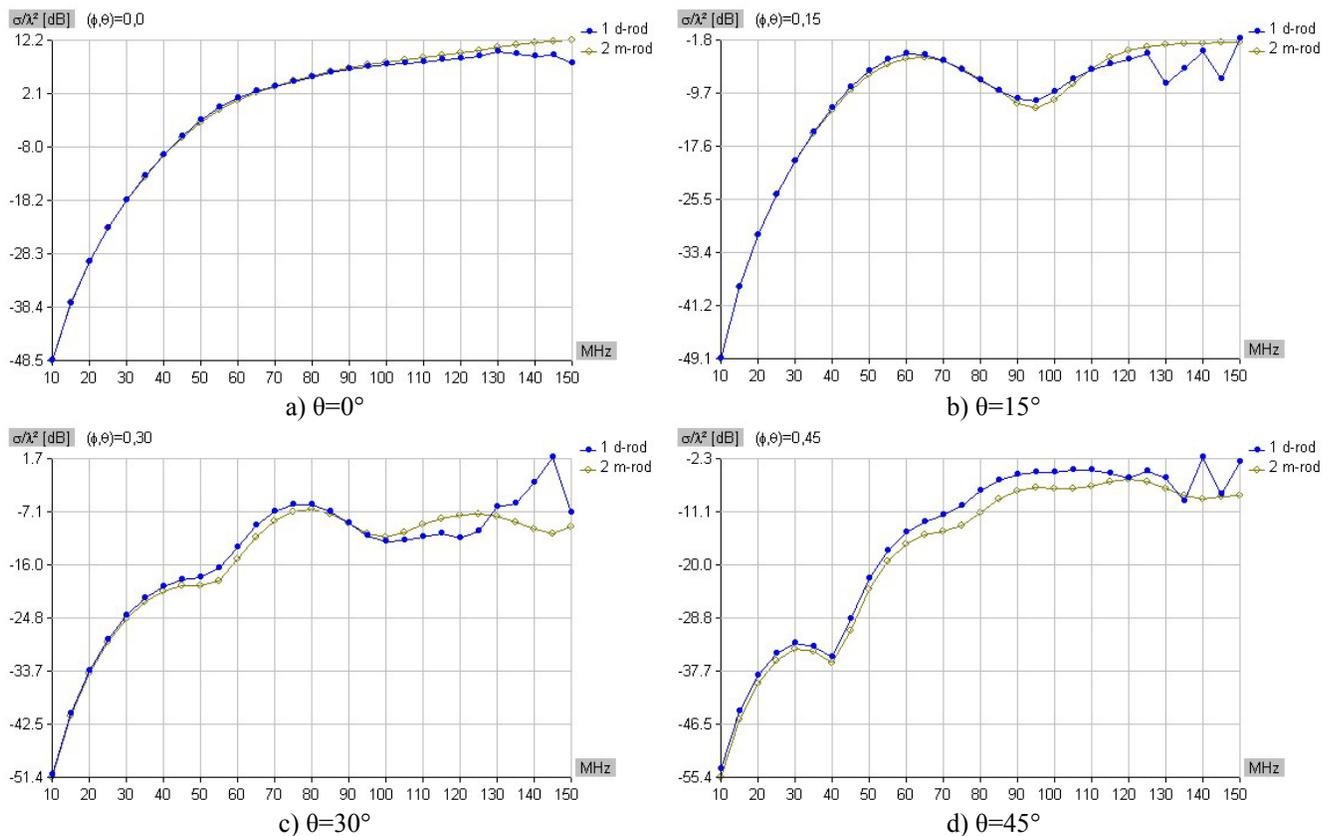
Figure 1. Monostatic RCS for dielectric rod and its approximation with metallic wire with distributed loadings.
