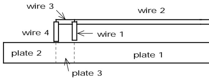
Figure 2 Segmentation of antenna elements and conducting plate #1.
