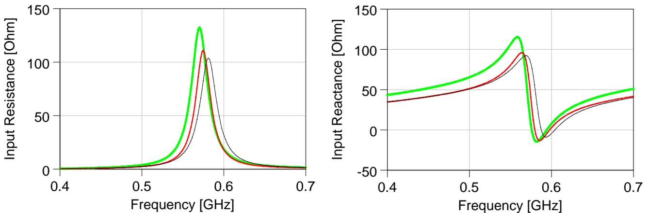
Figure 3 Calculated input impedance characteristics.
