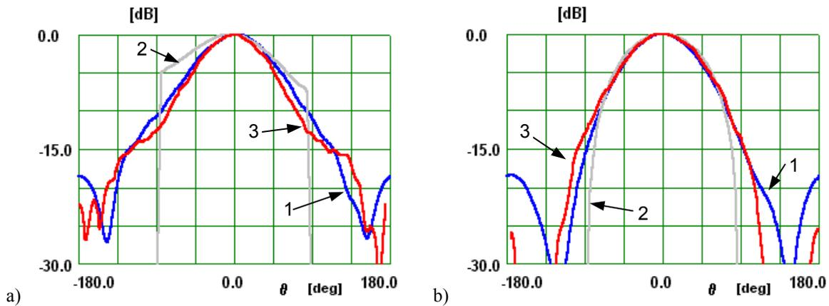
Figure 4 – Radiation pattern of irregular patch on thin substrate. 1 (blue): WIPL-D; 2 (grey): ENSEMBLE with infinite ground plane; 3 (red): measured. (a) E-plane; (b) H-plane
