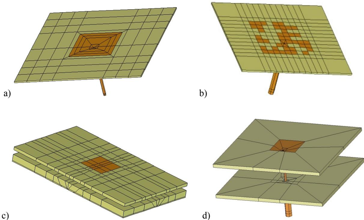
Figure 1 – Printed antenna configurations used for EM code assessment. A) Coaxial probe fed rectangular patch printed on thin substrate; b) Irregular shape patch printed on thin substrate; c) Double layer aperture coupled microstrip line fed rectangular patch; d) Rectangular patch printed on a thick substrate.
