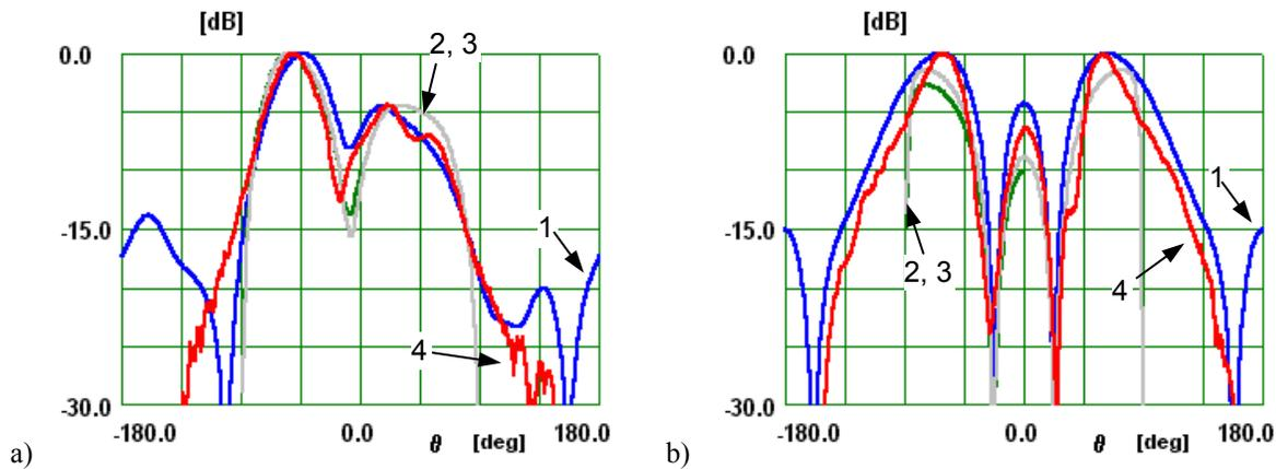
Figure 6 - Radiation pattern of thick patch. 1 (blue): WIPL-D; 2 (green): IE3D with infinite ground plane; 3 (grey): ENSEMBLE with infinite ground plane; 4 (red): measured. (a) E-plane; (b) H-plane
