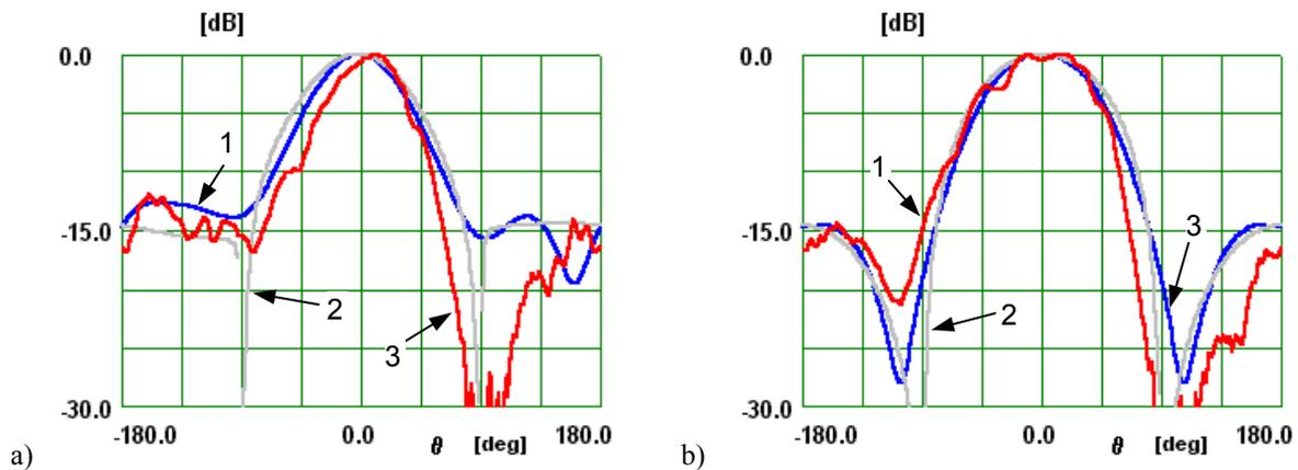
Figure 5 – Radiation pattern of double-layer wideband patch. 1 (blue): WIPL-D; 2 (grey): ENSEMBLE with infinite ground plane; 3 (red): measured. (a) E-plane; (b) H-plane
