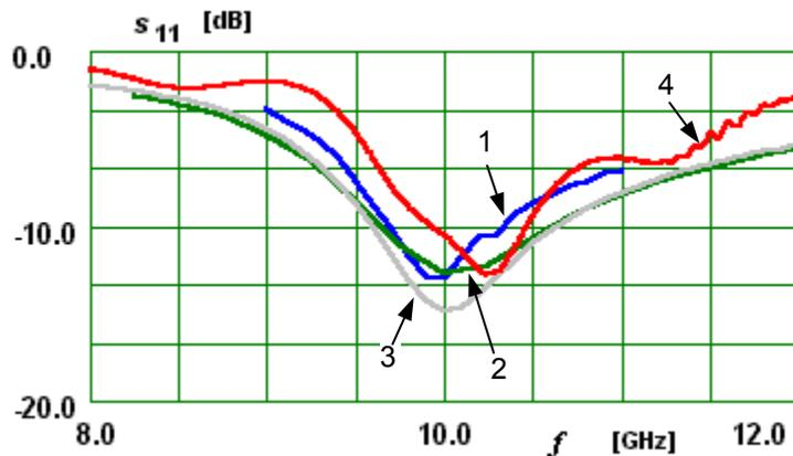
Figure 7 - Return loss of thick patch. 1 (blue): WIPL-D; 2 (green): IE3D with infinite ground plane; 3 (grey): ENSEMBLE with infinite ground plane; 4 (red): measured.
