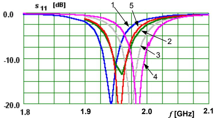
Figure 3 – Return loss of rectangular patch on thin substrate. 1 (blue): WIPL-D; 2 (green): IE3D with infinite ground plane; 3 (grey): ENSEMBLE with infinite ground plane; 4 (magenta): ENSEMBLE with finite ground plane; 5 (red): measured.
