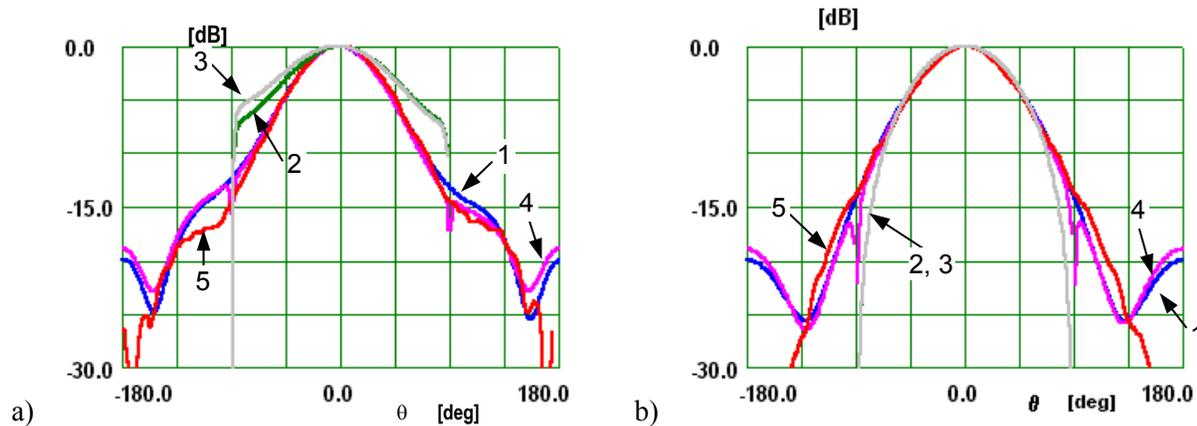
Figure 2 – Radiation pattern of rectangular patch on thin substrate. 1 (blue): WIPL-D; 2 (green): IE3D with infinite ground plane; 3 (grey): ENSEMBLE with infinite ground plane; 4 (magenta): ENSEMBLE with finite ground plane; 5 (red): measured. (a) E-plane; (b) H-plane.
