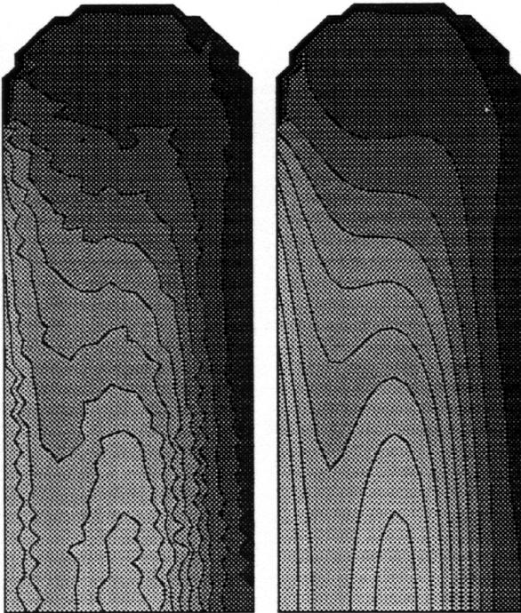
Figure 5: FE/MMP solution of the field in the cylinder (left) and the pure MMP solution (right), sampled on a regular 20 by 50 grid. The specific absorption rate is shown in the  $x$ - $z$  plane with the same scaling for both solutions; the higher the absorption, the lighter the color. A plane wave is incident from the left.
