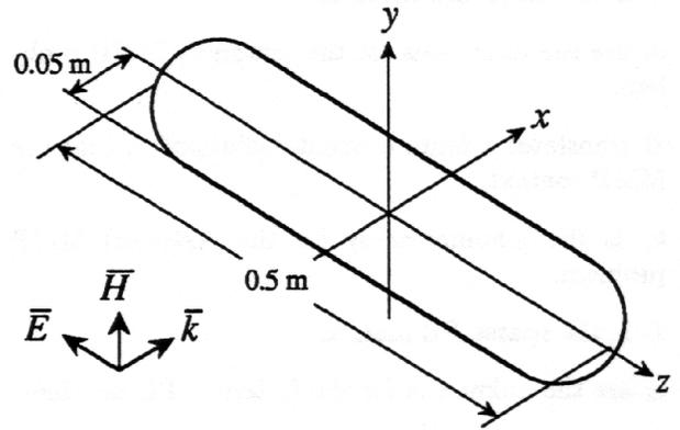
Figure 3: Geometry of the cylinder with spherical ends.
