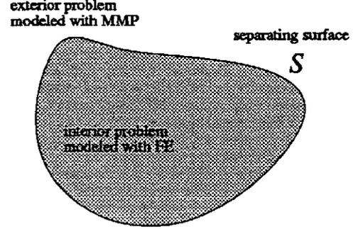
Figure 2: Separation of a problem into an interior and an exterior problem.
