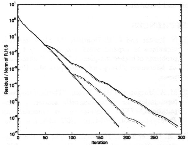
Figure 6: Residual as a function of iteration step for the pure FE problem (lines) and for the mixed FE/MMP algorithm (dotted line). Versions without restart, with a restart every 100 steps and with a restart every 50 steps are shown.
