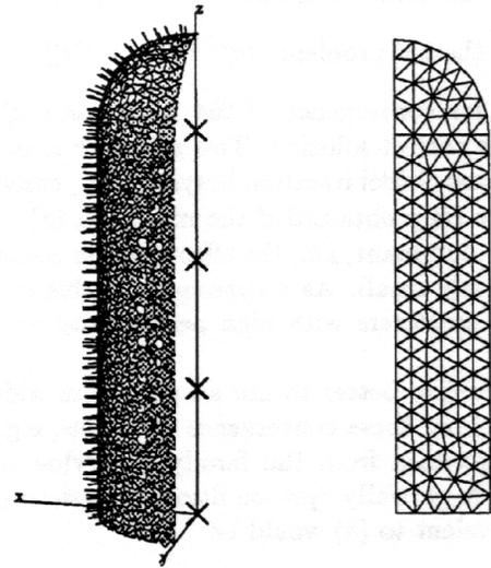
Figure 4: Surface discretization with matching points and location of the multipole expansions (left) and cut through the tetrahedral FE mesh in the  $z$ - $x$  plane (right). Thanks to the symmetry of the problem the scatterer needs to be discretized only in the first octant.
