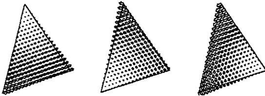
Figure 1: Vector basis functions  $\bar{W}^{12}$ ,  $\bar{W}^{23}$ , and  $\bar{W}^{31}$  for a triangular element, which are associated with the tangential value of the field along the corresponding edge.
