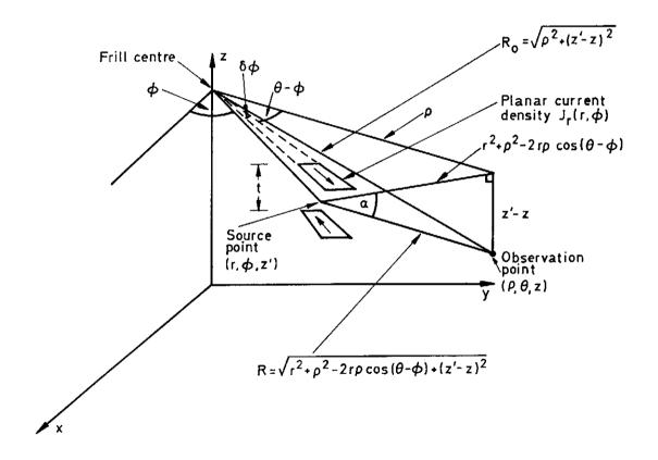
By the nature of the current sheets producing the frill, the direction of these currents are radially inwards and outwards respectively with respect to the frill centre. At the observation point, the contributions to the magnetic vector potential due to this elemental source are  $\delta A_{\rho}$  and  $\delta A_{\theta}$  in the radial and tangential directions respectively. With reference to the following figure:
