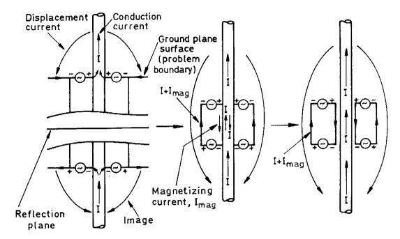
This arrangement now looks like a balanced antenna driven by a 1-turn toroidal transformer. There is still an annular ring of alternating magnetic flux (ie magnetic current), but the origin of this is easier to appreciate. It arises from a sheet of electric current flowing as the transformer primary. However, recalling the elementary theory of transformers, it is necessary to note that the total current flowing in this sheet comprises two parts:
