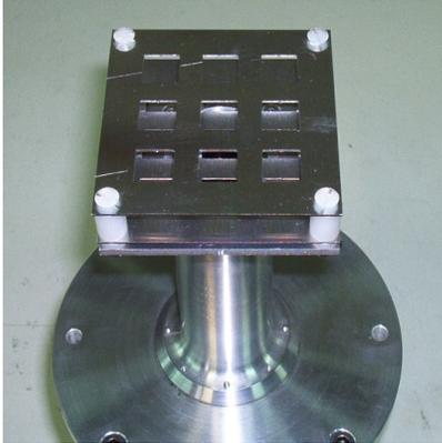
Fig. 3. Prototype of the EBG antenna.
