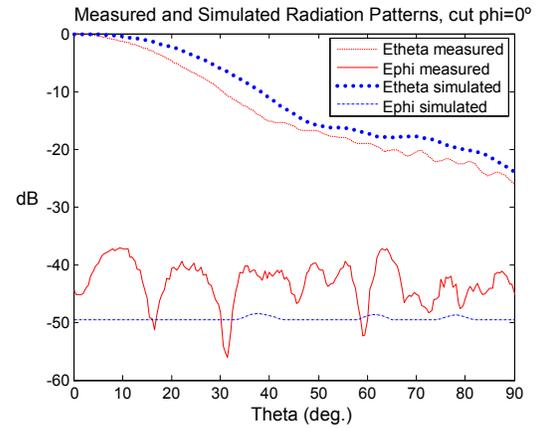
Fig. 4. Comparison of the simulated and measured radiation patterns. E-plane cut at 9.1GHz.
