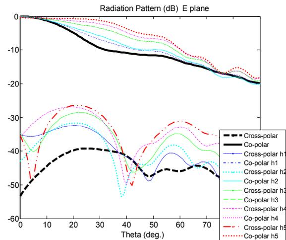
Fig. 9. Comparison between the simulated E-plane cuts at 9.0 GHz for several values of the height of the lower grid. The results for the optimum configuration are depicted in thick lines.
