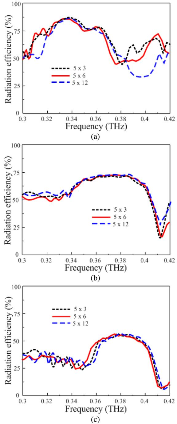
Fig. 3. Antenna radiation efficiency with different numbers of patch cells and different substrate thicknesses: (a)  $H = 80 \mu\text{m}$ , (b)  $H = 40 \mu\text{m}$ , and (c)  $H = 20 \mu\text{m}$ .
