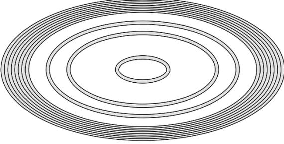
Fig. 5. Planar concentric coil with  $N_{ext} = 8$  and  $N_{int} = 3$ .
